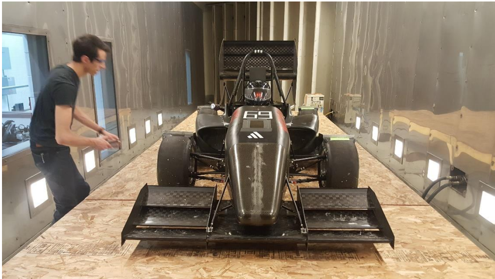
The racecar is placed onto four scales even with the platform. The goal here is to develop numbers relative to the CFD to prove the simulations are on track.
