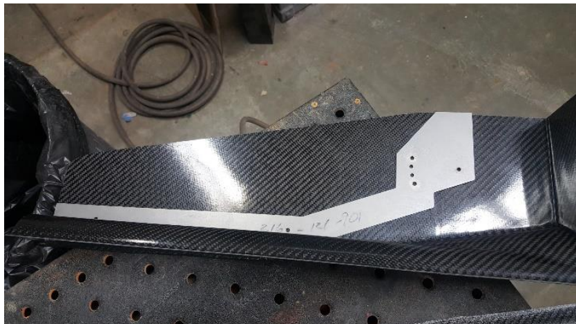
This is the endplate assembly jig. The holes are lined up and drilled out. All the different trim settings are on the jig.
