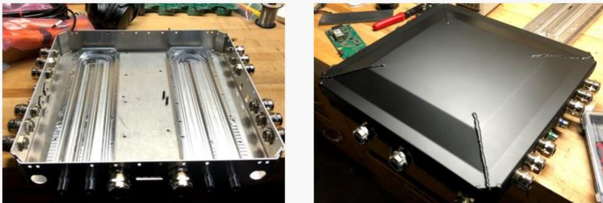
Figure 68: Inverter case with cold plates (left). Inverter cover (right)
