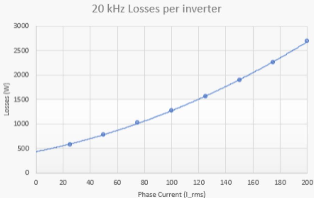
Figure 5: Power losses (Watts) vs. Phase Current ( $A_{RMS}$ ) at 20kHz switching frequency
